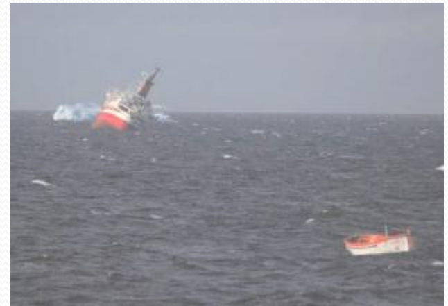
MV Explorer sank after being holed by bergy bit collision
